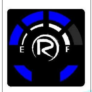
E. 2 lower blue led lights ON – permanent state with 3 blue led lights indicating LPG level ON – permanent state
