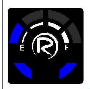
C. 2 lower blue led lights ON with 1 blue led light indicating LPG level ON – permanent state
