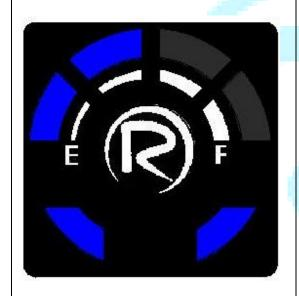
D. 2 lower blue led lights ON -permanent state with 2 blue led lights indicating LPG level ON - permanent state
