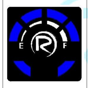
F. 2 lower blue led lights ON- permanent state with 4 blue led lights indicating LPG level ON- permanent state
